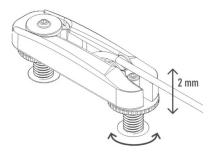
Tighten the Rear Saddle Lock-Down so it secures the Saddle.
