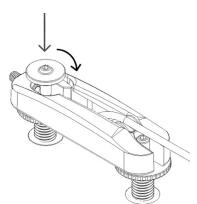
Install the string into the machine head, making sure the string is lying on the String Ramp Insert. Tune the string to pitch.
