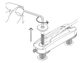
Lift Saddle off the Front and Rear Posts. Proceed to adjust height of posts. Post heights should be even at desired height.
