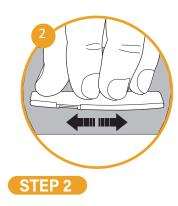
Check if the Graph Tech saddle fits into the slot, without forcing it. If it's too thick, place a 240 to 400 grit sand paper on a flat surface and sand the sides of the saddle until it fits in the slot snugly but is easily removable. You may have to reduce the length also.
