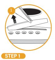
**Remove the strings and bridge pins.** The saddle should lift out easily. If you find it is glued in, get a competent guitar tech to complete the replacement. DO NOT pry it out as you may take some wood from your bridge with it. Once removed, clean the slot of any debris.
