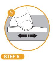
Sand the bottom of the saddle up to the line, keeping the bottom flat and square to the sides. Work in small increments and check your work frequently so you don't remove too much material.
