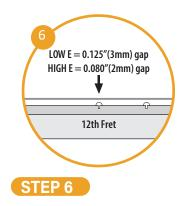
**Determine correct string height**, by measuring the gap between the top of the 12th fret and the bottom of the low E string. It should be around 0.125" (3mm), or about a stack of 12 business cards if you don't have a ruler. For the high E string, the gap should be around 0.080" (2mm), or about a stack of 8 business cards.
