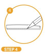
**Adjust the string height.** Put your old saddle against the GraphTech saddle and align the tops. Using a pencil mark a line along the bottom of your new saddle.
