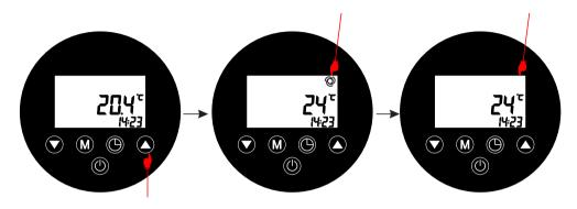
1.Long press 3s to turn on pump. 2.Long press 3s again to turn off pump.
