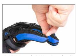
Fig. 32 Reattach DIP Tensioner for all fingers.
