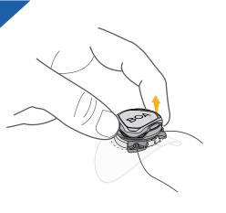
Pull dial outward to disengage spool.
