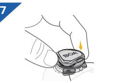
Ensure that the dial is pushed in to engage the spool, then wind the laces by twisting the dial
