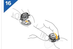
Re-insert cartridge into base by putting the bottom tab in first, then clicking the cartridge into place.
