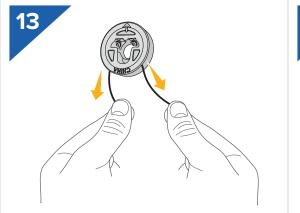
Pull the lace back through the spool so the knots are secured in the middle of the spool. The knots should not come out of the top of the spool.
