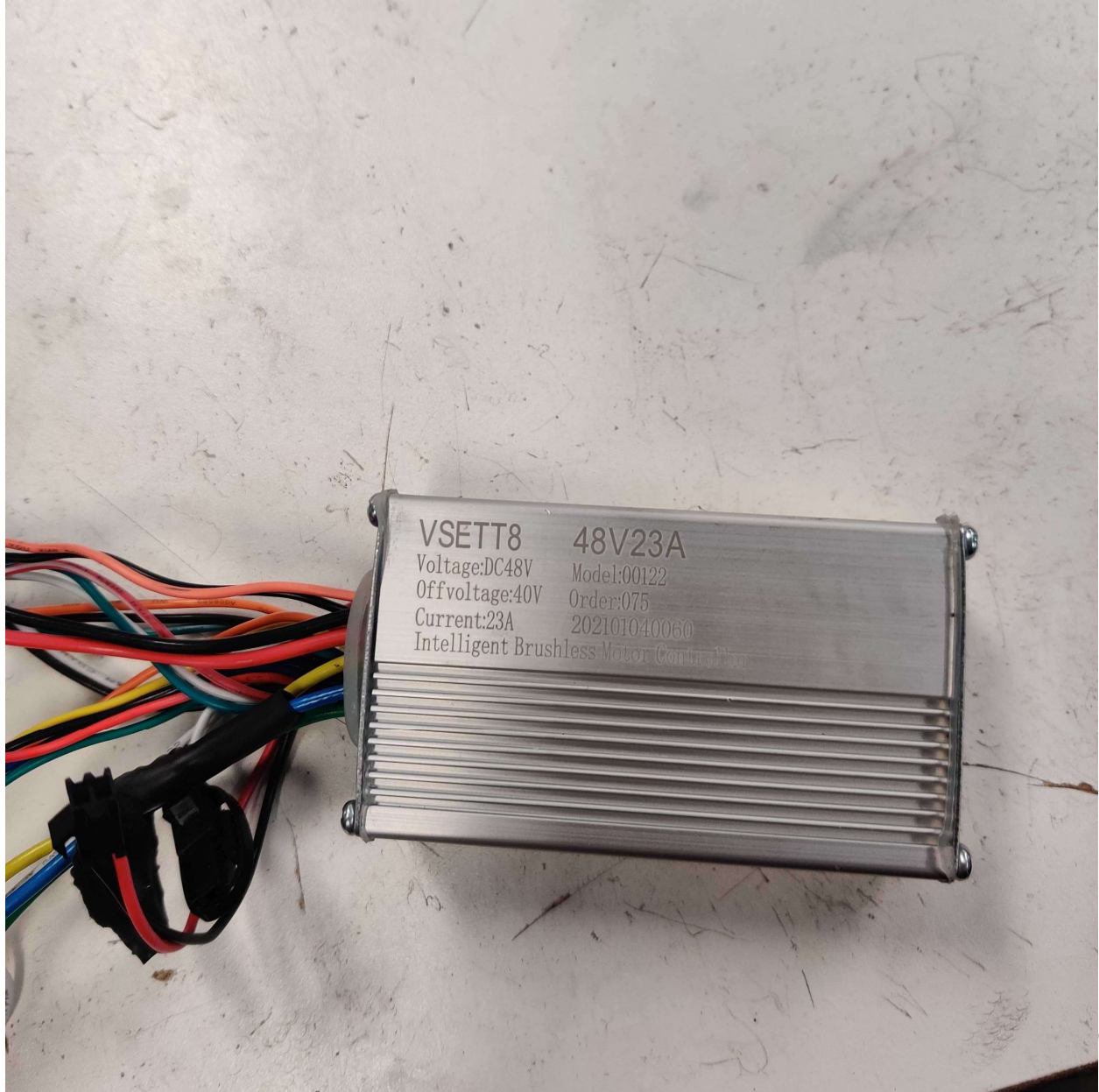
Figure 2a: Motor controller
