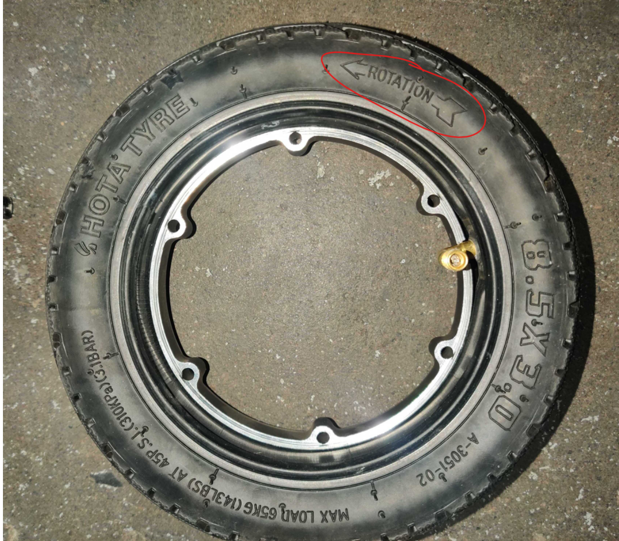
Figure 3b: Split rim / tire tread rotation arrow
