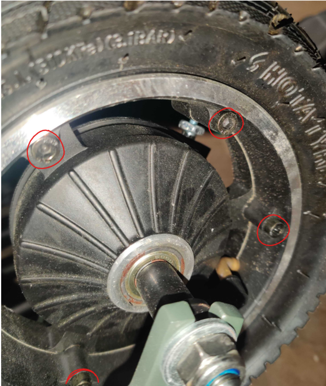
Figure 3a: rim screws – note your configuration may be slightly different based on process / model revision
