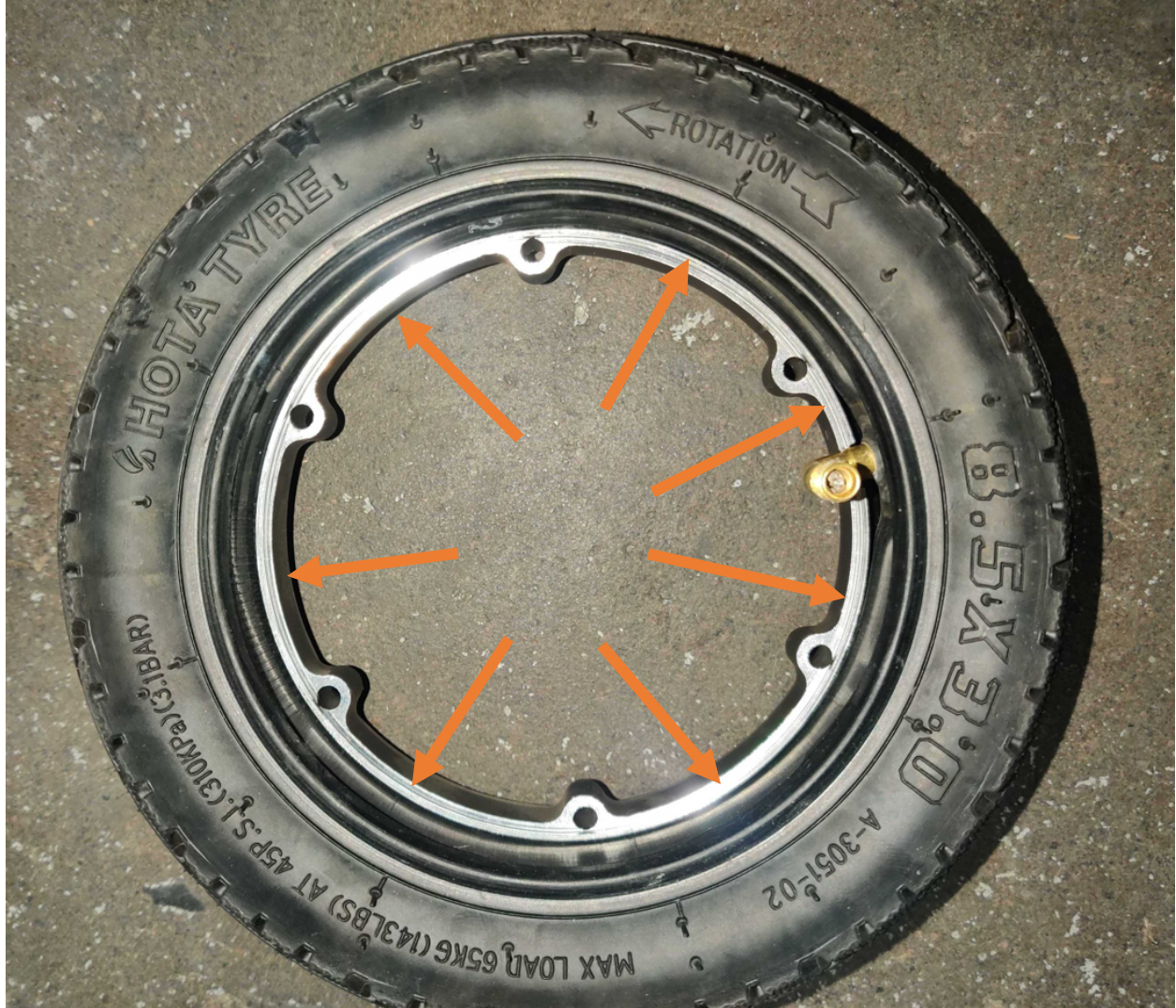
Figure 4a: Inner tube seating
