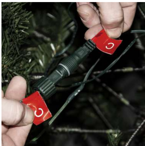
6. Attach cables C-C before connection the transformer to the new foot pedal cable. Once wires are connected and in place - Plug in transformer to check everything is working.
