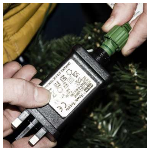
6. Attach cables C-C before connection the transformer to the new foot pedal cable. Once wires are connected and in place - Plug in transformer to check everything is working.
