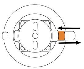
Pump each SeaSucker repeatedly until the plunger doesn't spring back and the indicator band is hidden inside the pump cylinder. If the plunger won't stay seated in the pump cylinder or continues to extend out immediately after pumping, you may need to clean the mounting surface or the vacuum pad or pump, perform basic maintenance on the vacuum pad or pump, or move to a more suitable mounting position. Do not use your Heavy-Duty Antenna Mount without correcting the problem!
