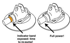
To get the most out of your vacuum mounts, inspect them regularly and store them with the vacuum mounts' protective covers on. Check that all screws are securely tightened, including the screws attaching the vacuum pads to the SeaSucker housing and the screws attaching the SeaSuckers to the mounting deck.
