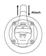
It may help to moisten the bottom edge of each vacuum pad with water - do not use cleaners, lubricants or other liquids.
