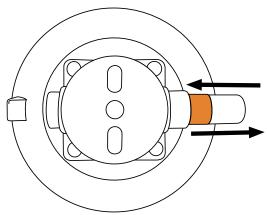
Pump each SeaSucker repeatedly until the plunger doesn't spring back and the indicator band is hidden inside the pump cylinder. If the plunger won't stay seated in the pump cylinder or continues to extend out immediately after pumping, you may need to clean the mounting surface or the vacuum pad or pump, perform basic maintenance on the vacuum pad or pump, or move to a more suitable mounting position. Do not use your Auxiliary Light Mount without correcting the problem!
