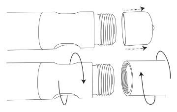
Now line up the threaded connector with the open bar end and thread the two pieces together. Continue until the threaded connector is fully seated in the bar (it should look like the other side that came preassembled from the factory). Give the bars a firm twist to complete the assembly - nothing more than hand pressure should be needed to make a secure connection. Repeat for the second bar.
