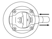
Clean the surface you're going to attach the mount to. Dust and dirt will affect the vacuum mount's ability to create and hold vacuum. Remove the protective cover from each vacuum mount and inspect the rubber vacuum pad for damage or dirt. Do not use a vacuum mount with any visible damage to the vacuum pad. If the vacuum pad is dirty, clean it with a mild soap and water solution and a soft cloth or sponge.
