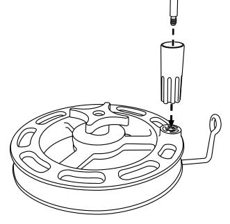
Press the vacuum pad firmly against the mounting surface to make a full seal. Pump repeatedly until the plunger does not spring back and the indicator band is hidden inside the pump cylinder. If the plunger won't stay seated in the pump cylinder or continues to extend out immediately after pumping, you may need to clean the mounting surface or the vacuum pad or pump, perform basic maintenance on the vacuum pad or pump, or move it to a more suitable mounting position.
