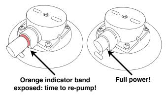
or abrasive cleaning pads. If the pump feels sluggish or obstructed, pull the plunger straight out of the pump and clean any dirt out of the inside of the pump. Clean the plunger's black rubber gasket and lubricate the gasket with silicone gel (our recommended lubricant, Lube Tube, is available on-line at www.seasucker.com). Do not use petroleum-based lubricants on the gasket. Insert plunger back into the pump cylinder and push in until seated normally.
