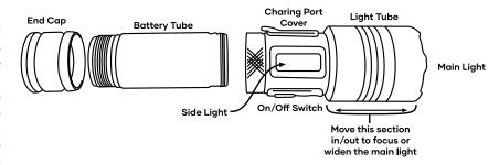
Press the on/off button one time to turn on the main light. Additional presses will dim the main light, strobe the light, or turn it off. You can also turn off the light by pressing and holding the on/off button. Rapidly press the on/off button twice to turn on the side light. Additional presses will dim the light, change it to a red light, strobe the red light, or turn it off.
