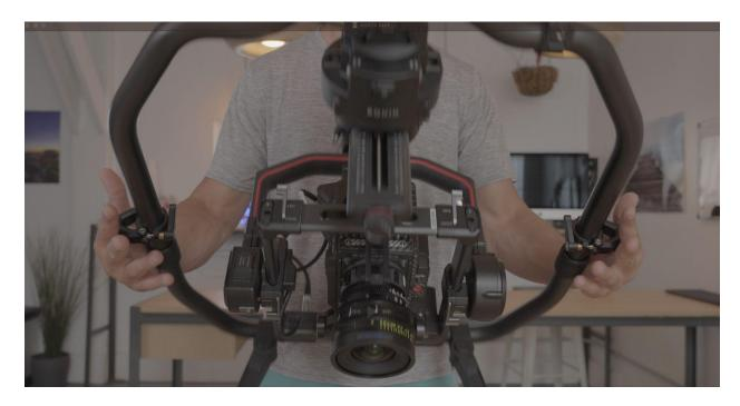
To fix this, slightly loosen the clamps and move the Quick Connect Clamps up.
