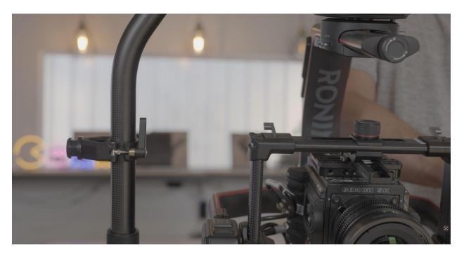
To get started balancing the vertical tilt, put your hands under the Quick Connect Clamps with the clamps resting on top of your hands and grip the gimbal ring. Slightly release your grip on the ring to let the gimbal freely rotate.
