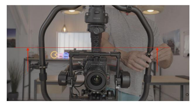
If the Ready Rig Quick Connect v2 clamps are mounted **too high**, the gimbal will feel like it wants to settle in the correct orientation but tilting the camera up and down will feel difficult due to the camera's weight acting like a pendulum.
