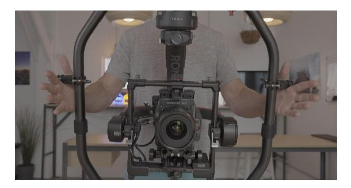
If the Ready Rig Quick Connect v2 clamps are mounted *too low*, the gimbal will want to flip upside down.
