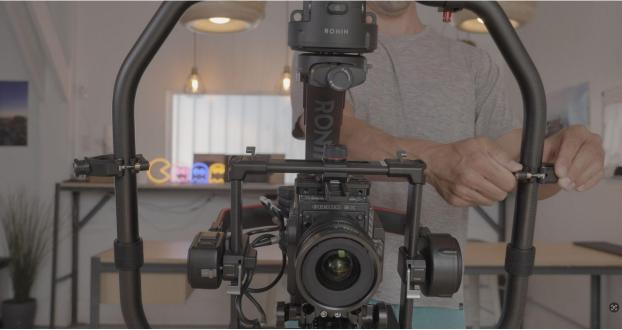
If the *gimbal falls away from you* as you hold it, <u>slightly loosen</u> the Quick Connect's lever and *rotate the Quick Connect Clamps away from yourself* and retighten.
