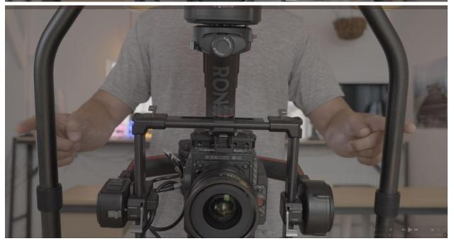
Step 3 — Attach your Quick Connects to the imaginary line and tighten down the lever clamps
