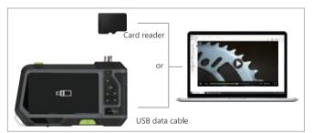
You can use a TF card reader to copy data directly or use a USB cable to connect to a computer for copying.
