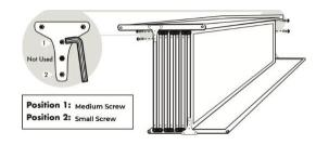
Line up bracket on end panel to the holes on the outside piece of panel bundle. Screw two bolts into each bracket on the end of the panels as shown.
