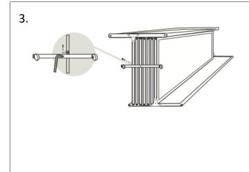
Screw wheel base to bottom of panels into square nuts. Image shows approximate placement. The bottom of panels are predrilled.
