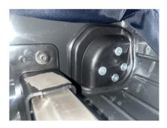
Align and insert the new wheels and screw the existing screws in place and re-zip the lining
