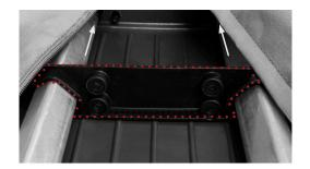
Insert the new handle system and ensure the metal pipes are going through the black bracket.
