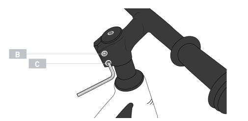
**Note:** alternating is important because as you tighten one side bolt you cause the other bolt to be able to be tightened further. Both these bolts must be tightened **fully**.
