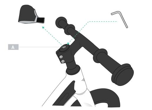
3. Remove the protective neoprene cover and use the 5mm Allen key provided to adjust the top bolt **A**. It should be finger tight (to eliminate play in the headset). Be careful not to overtighten as it should not restrict the steering: the handlebars should turn freely. Overtightening will damage the bearings.
