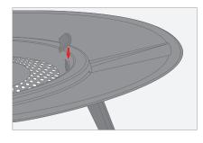
05. After pushing down, press the **cap** in toward the perforated grate.
