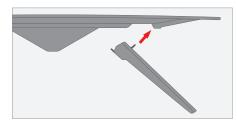
02. Push the **upper tab** into position by pressing inward at the bottom of the leg.
