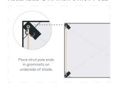
Use strut pole if mounting MoonShade to anchor points less than 7 feet apart.
