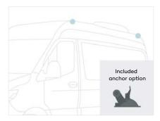
It's very important that your anchor points are secure! If using suction cups, be sure to wipe the surface clean first and make sure they're securely attached before proceeding.
