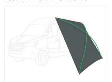
Assemble tension and support poles. Place tension poles in corner pockets diagonally across MoonShade and attach clips.
