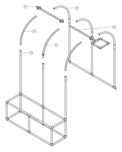
NOTE: THE WATER HOLE ON PART (J) SHOULD FACE DOWNWARDS.
