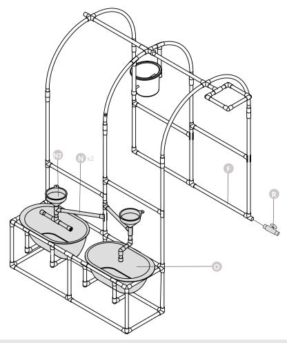
IMPORTANT: PLEASE ENSURE THAT ALL CONNECTIONS ARE TIGHT BEFORE ATTACHING A HOSE. IF WATER LEAKS OCCUR, YOU WILL NEED TO TIGHTEN THE CONNECTIONS BY PUSHING THEM TOGETHER OR USING A RUBBER MALLET TO BANG THEM CLOSED. AFTER ATTACHING THE HOSE, OPEN THE WATER SLOWLY. YOU CAN ADJUST THE SPRINKLER FLOW BY LOWERING AND RAISING THE WATER
