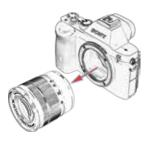
Remove the lens from the Sony E-Mount interchangeable lens camera by depressing the lens release on the front of the camera, turning the lens counter clockwise until end orientation marks are aligned, then pull the lens away from the camera body. Keep lens away from the camera body. Keep to protected with a rear lens can.
