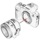
While the Sony E-Mount camera is turned off, install the Canon lensif ISION assembly by install the Canon lensif ISION assembly to the adapter and font of the camera, inserting the adapter and font of the camera, inserting the adapter into the camera's lens mount then turning lockwise until you here a click which indicates the assembly is safely locked into place on the camera.
