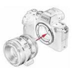
While the Sony E-Mount camera is turned off, install the lens / adapter assembly by lining up the orientation marks on the rear of the adapter and front of the camera, inserting the adapter into the camera's lens mount then turning clockwise until you here a click which indicates the assembly is safely locked into place on the camera.
