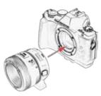
While the Micro Four Thirds camera is turned off, install the lens/FUSION assembly by lining up the orientation marks on the rear of the adapter and front of the camera, inserting the adapter and front of the camera is ens mount then turning lockwise until you here a click which indicates the assembly is safely locked into place on the camera.
