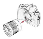
Remove the lens from the Micro Four Thirds interchangeable lens camera by depressing the lens release on the front of the camera, turning counterclockwise until the orientation marks are aligned, then pull the lens away from the camera body. Keep the rear optic of your Micro Four Thirds lens protected with a rear lens can.
