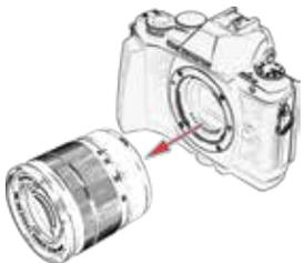
Remove the lens from the Micro Four Thirds interchangeable lens camera by depressing the lens release on the front of the camera, turning counterclockwise until the orientation marks are aligned, then pull the lens away from the camera body. Keep the rear optic of your Micro Four Thirds lens protected with a rear lens cap.
