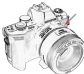
Included on the adapter is an 'Iris Toggle' switch which supports aperture control through the adapter for select cameras that do not allow for in-camera aperture control. You can adjust the aperture from the adapter to directly control the lens actual aperture.
