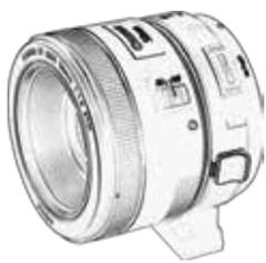
Mount your lens onto the Fusion adapter by lining up the orientation marks (red dot for EF lenses, white square for EF-S lenses), inserting the lens into the front of the FUSION adapter and turning clockwise until you hear a click. To remove the lens from the adapter, slide the lens release tab on the side of the adapter away from the lens, turn the lens counterclockwise until the orientation marks are aligned, then slide the lens out of the adapter.
