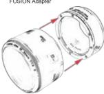
Mount your lens onto the Fusion adapter by lining up the orientation marks (red dot for EF lenses, white square for EF-S lenses), inserting the lens into the front of the FUSION adapter and turning clockwise until you hear a click. To remove the lens from the adapter, slide the lens release tab on the side of the adapter away from the lens, turn the lens counterclockwise until the orientation marks are aligned, then slide the lens out of the
