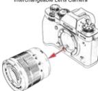
Remove the lens from the FUJIFILM X Series interchangeable lens camera by depressing the lens release on the front of the camera, turning counterclockwise until the orientation marks are aligned, then pulle lens away from the camera body. Kep the rear optic of your Fujinon X Mount lens protected with a rear lens cap.
