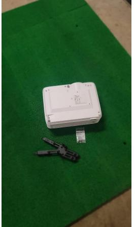
Step 3: Extend one of the arms by undoing the hexscrew on top and then redoing it into the 2nd hole in the arm to extend it further.
