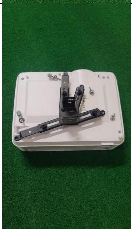
Step 5: Insert the screws and washers to attach the arms to the projector. Step 6: Ensure all screws are tightened to secure the projector.
