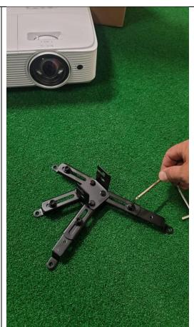
Step 4: Undo the soft-tipped screws (x2) and prepare the 2 screws from the plastic sleeve. Layout the 4 arms as per below photo to be ready to attach the projector.
