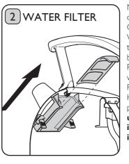
Make sure the appliance is switched off, unplugged and allowed to cool. Open the Lid. Hold the top of the Water Filter, pull up and out of the kettle. Rinse under a tap whilst brushing carefully with a soft brush. Rinse out the kettle with fresh water. To replace align the Water Filter with the grooves in the Filter Holder, insert and push back into place. Do not operate kettle unless water filter is correctly in position. Risk of scalding and injury caused by misuse.
