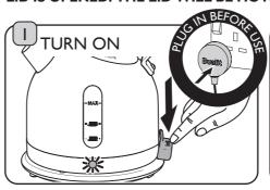
Plug the kettle into the power socket. Press the 'On/Off' switch down. The power neon will illuminate and the kettle will start to heat up. If the kettle is accidentally switched on with no water inside, the boil-dry device will switch off the heating element to prevent damage to the kettle.
