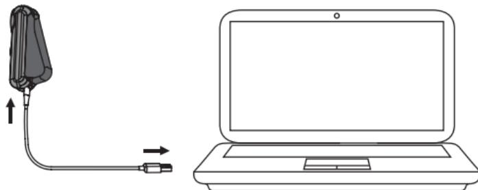
**Note:** The time to charge from flat to fully charged varies from 3 to 6 hours depending on method of charging i.e. mains power USB (not supplied) or computer USB
