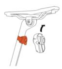
You can easily remove Fly6 CE from your bike by removing it from the seat post mount with a 1/8<sup>th</sup> turn. You can leave the mount on your bike for next use.
