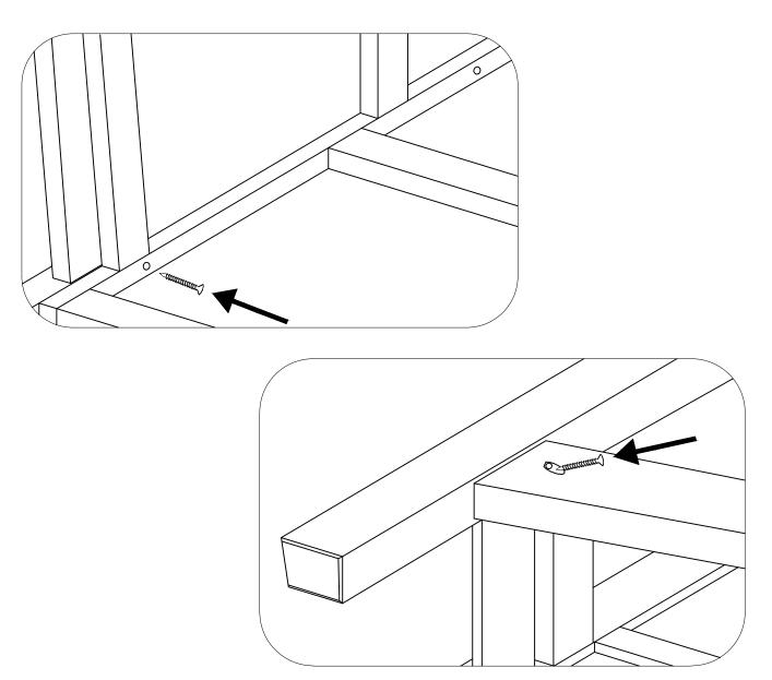
STEP 10 Attach the top using Dowel (  $8 \times 30$  ) and screw C (  $4 \times 30$  )
