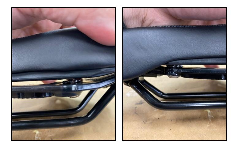
Please note that with the wedges, it is the same process, but the grip washers will go on the top of the wedge versus the frame.
