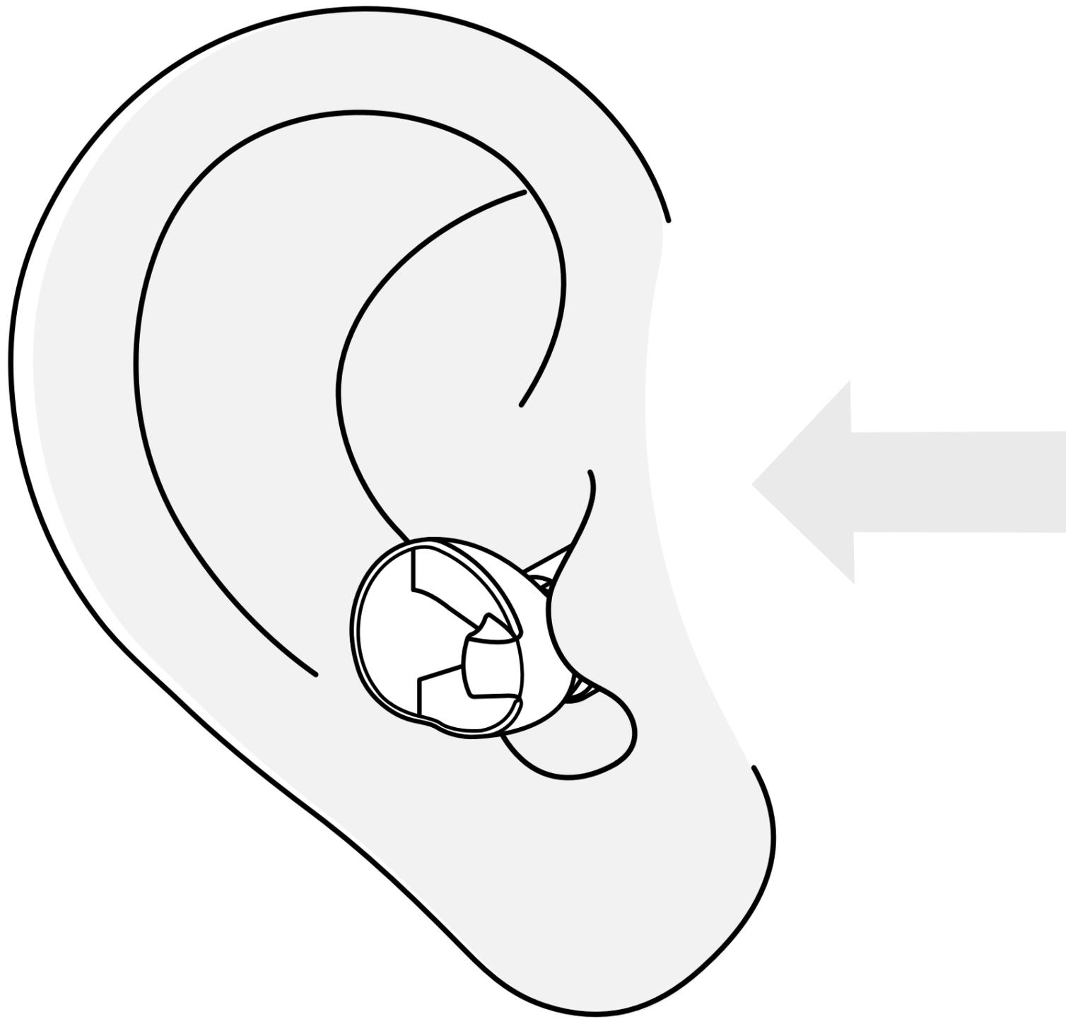
Definition should be fitted **horizontally** and not pointing upwards or sticking out of the ear.
