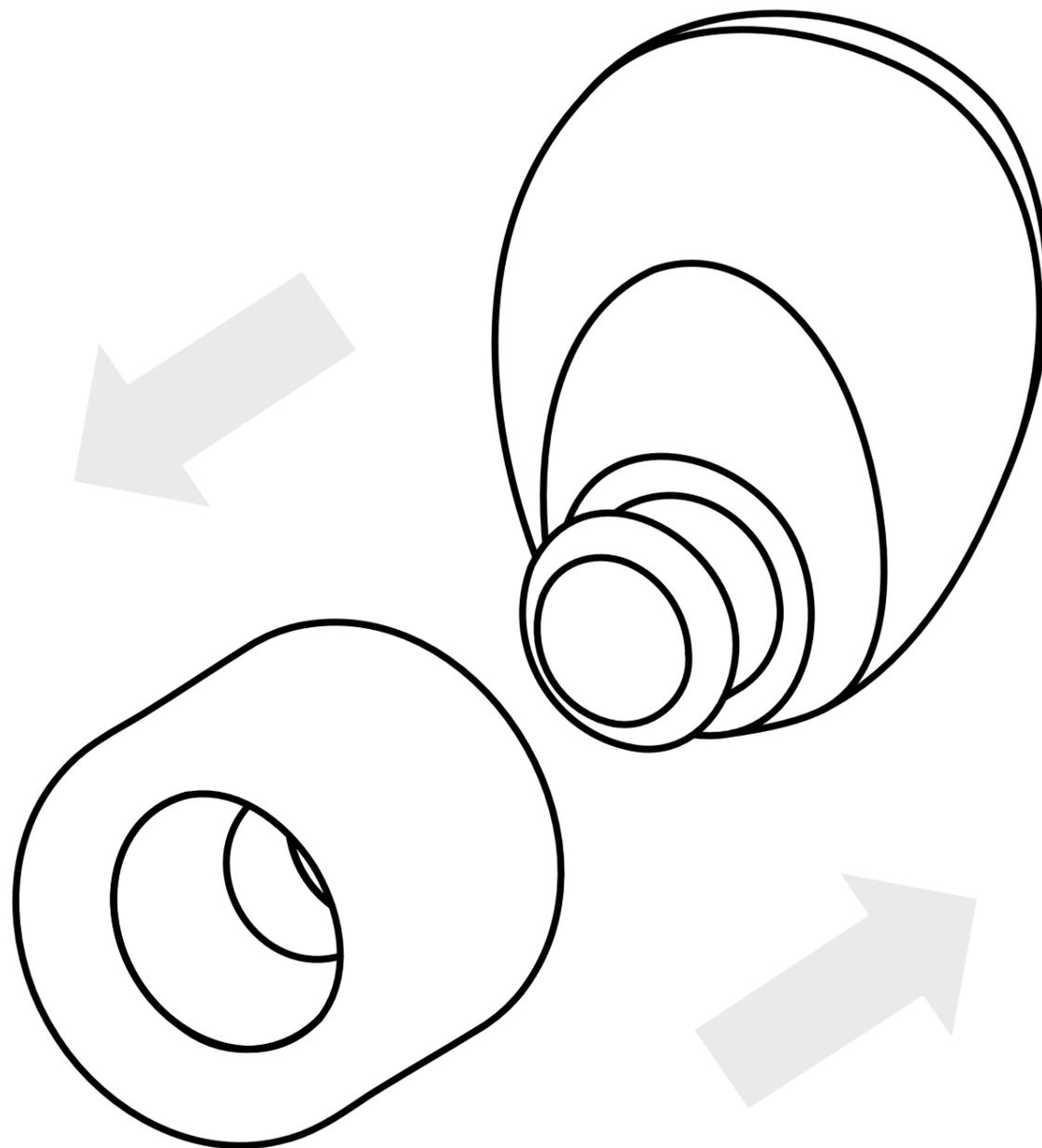
Select a suitable tip size (if you are unsure, start with the smallest tip) and attach it to the body.
