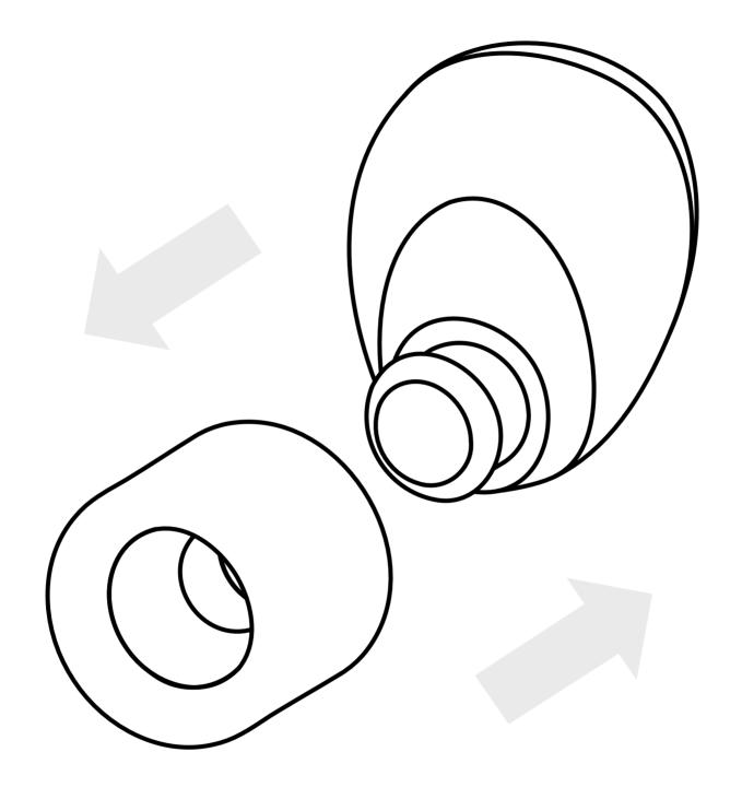
Select a suitable tip size (if you are unsure, start with the smallest tip) and attach it to the body.
