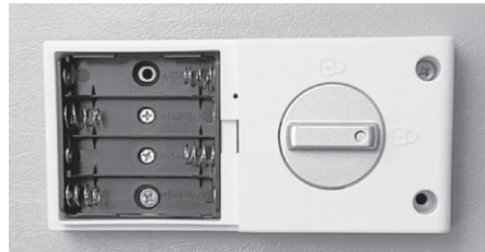
H: Control box (battery cover removed)
