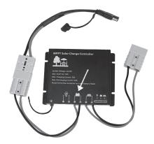
On the charge controller, you should see the middle indicator light turn green. This means the battery is connected. Steady green is normal. If it's flashing, see the TROUBLESHOOTING table on page 6.
