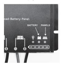
The series of five green lights below that indicate the approximate voltage being produced by the battery.
