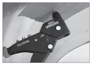
**NOTE:** You must hold the rivet tool firmly against the wall while simultaneously squeezing the handle of the tool. Each pump of the rivet tool will become tighter each time. Don't let the rivet slide out while you are squeezing. (This takes a bit of practice, but you'll get the hang of it quickly.)
