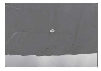
Pull the tool away and admire your handiwork. The rivet will have an empty hole in the center where the stem used to be, and you'll find that broken-off stem in the rivet tool. Just shake the stem out and you're ready to install another rivet.
