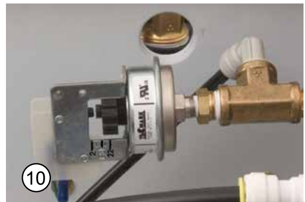
Low Pressure Switch shown set at 10 psi and is unpressurized
