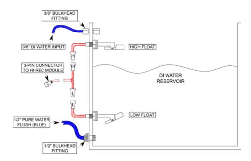
NOTE: Floats must be installed in a DI WATER storage container. This system MUST be connected to the floats to operate the Flush Cycle. Failure to install the pure water flush connection for this unit will void any warranty.
