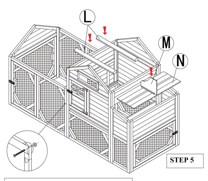
This rod allows you to open and close the door on the hen house from outside of the run. Connect the rod to the handle using the small screw and nut
