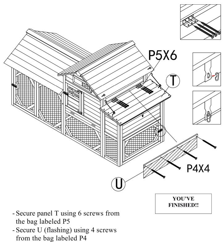
\*This flashing (piece U) should be installed just above where the nesting box roof lid connects to the hen house. This flashing will help keep the inside of the coop dry.
