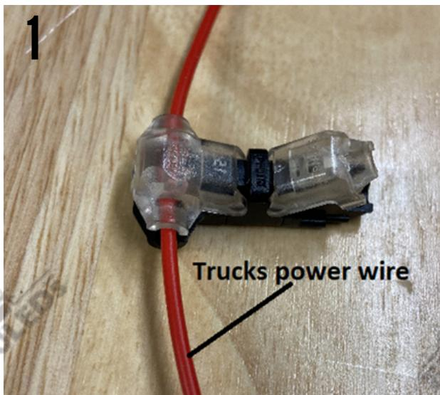
**Step 2: Insert the power wire from the F150LEDS.com kit into the hole in the opening seen in the image then use pliers and clamp the opening so the wire is securely connected**
