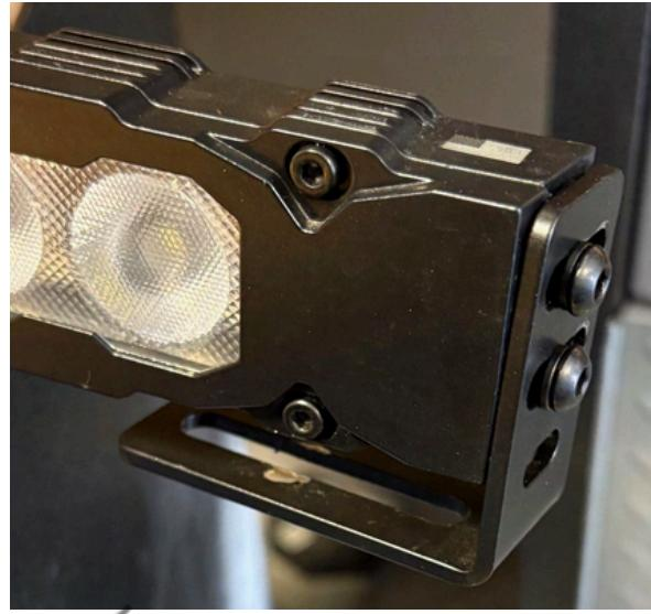
Put the hex head bolt down into the long channel under the bar.
