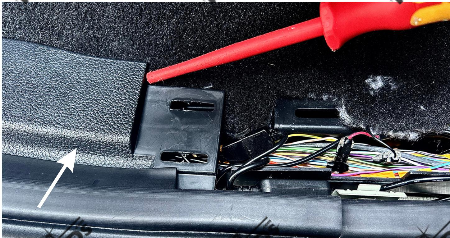
**\*\*We were able to gently lift this plastic trim to hide most of our power harness/wires underneath the plastic.**
