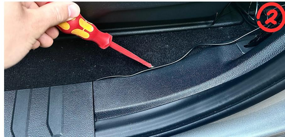
\*\*We used a flat head screwdriver to gently wedge the wire behind the plastic trim in order to make it easier to hide the wires.
