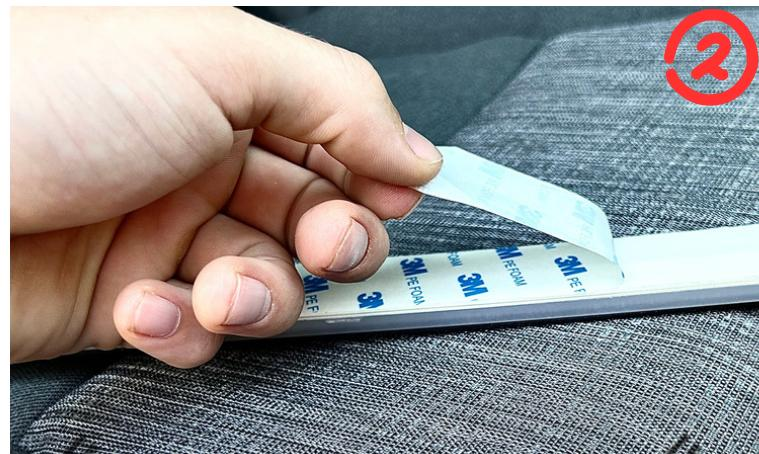
**Once the 3M tape has been removed, line up the door sill plate with the plastic trim cover and mount the plate to the truck.**
