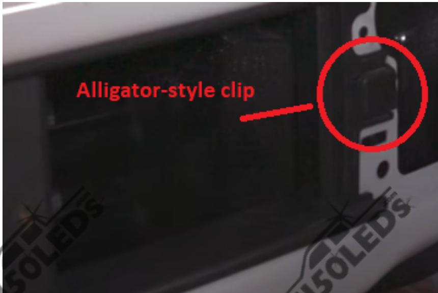
*\*It is helpful to reach behind the lower intake piece and pinch the alligator-style clips while pulling away from the truck\*.*
