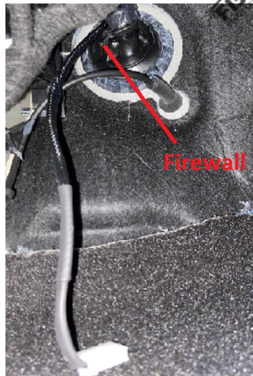
Now run the male connector from the switch in-between the steering wheel and the plastic piece seen in the photo below.
