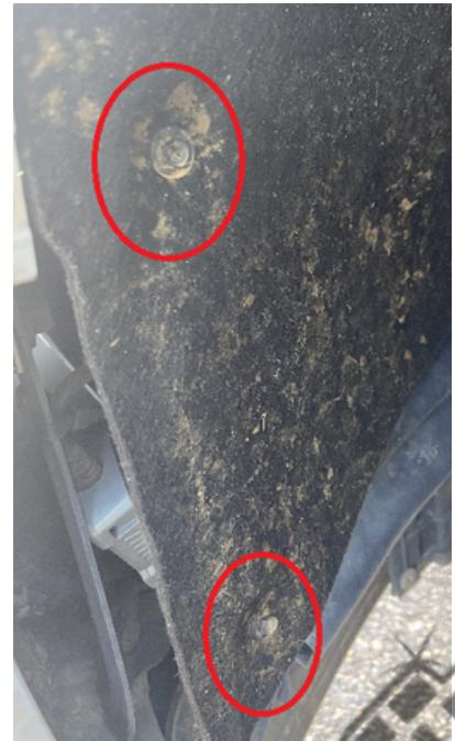
The first two screws are located right inside the wheel well, and the screw connecting the wheel well liner to the trim piece is at the top of the wheel well.
